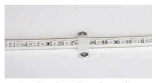
Place the strip on the surface and use a plastic clip to fix it. We recommend to use one clip every 3ft, and remember don't clip over the LED chips.
