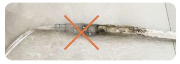
▲ Do not submerge the light in liquids. Connections are non-waterproof yet. Keep all connections away from water and moisture to prevent circuit damage which can lead to fires.
