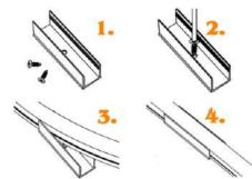
Or you can fix aluminum mounting clip or track on the wall using screws, and than insert the light strip into the clip or track.
